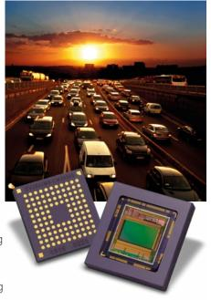
Motion free artefacts, miniaturization, low cost and low power, are all key characteristics that fuel the design of new (and future generations) of imaging systems. Teledyne e2v's new Emerald 2M CMOS image sensor offers an easy solution to all of these requirements by integrating on-chip functionalities that reduce the computational load on the processor as well as programming time for engineers.
